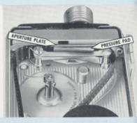
4 Place the spool of film on the supply spindle marked "Full Film Spool." The flange of the spool stamped "Kodak-8 Spool" must be uppermost. Make quite certain that the spool is properly seated—the end of the supply spindle should project through the hole in the spool flange.
