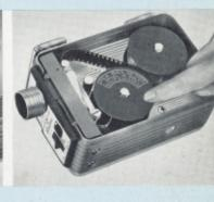
7 Hold the empty take-up spool as shown above. Fold the end of the film to form a quarter-inch hook, then hook this into the slot in the spool core; wind the slack film, black or shiny side out, on to the take-up spool by turning the spool in the direction of the arrow. If the spool is bent the film will bind; as a temporary measure carefully bend the flanges outwards. Renew the spool as soon as possible.
