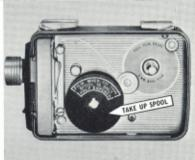
Never load the camera with the motor unwound. So first of all, give the winding key a few turns before you start to load. 2 Next, press in and slide the cover latch as far as it will go in the direction indicated to open. Lift off the cover.
