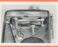
6 Push the film all the way down, at the top of the camera first; then at the bottom. Pull the film through the gate until there are approximately 9 inches below the gate.
