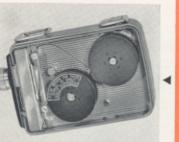
When the film is run through the camera the first time, only one side is exposed. To expose the other side, remove the empty spool, place the full spool on the supply spindle with the instructions down and rethread the film as described in the section on loading. Before rethreading, make sure the gate is free of dirt, pieces of film, or foreign particles.
