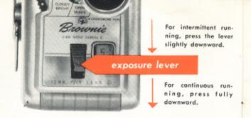
To start the motor of your Brownie Movie Camera, press the exposure lever slightly downward. To stop the motor, release the lever. When you press the ex-
