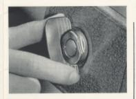
1 First of all, give the winding key a few turns before you start to load, to make sure that the motor is not run down. Never load the camera if the motor is run down.
