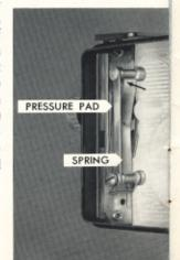
Carefully clean the polished surfaces of the gate and pressure pad with a slightly moist cloth; do not scrape the track with any metallic object. Then polish the parts with a clean, soft, lintless cloth. Make sure the parts are dry.
