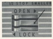
2 Next, press in on the center spring leaf of the cover latch (shown by the arrow in the picture above) and at the same time slide the latch as far as it will go in the direction indicated to open.
