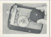
4 Place the spool of film on the supply spindle. The flange of the spool stamped "Cine-Kodak 8 Spool" must be up. Make sure that the spool is properly seated—the end of the supply spindle should project through the hole in the spool flange.
