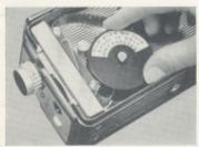
8 Place the spool on the take-up spindle so that the instructions are up. Turn the spool slightly, if necessary, so that the spool fits all the way down with the end of the spindle projecting through the hole in the spool.
