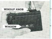
Close the back of the camera by pressing it against the camera body until it locks. The film name and number of exposures per cartridge appear in the winpow on the back of the camera. (When motor is wound, first exposure positions itself immediately.)
