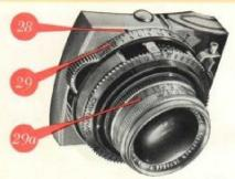
Set the distance in the same way as with the telephoto lens. Transfer the distance figure obtained with the rangefinder to the wide-angle distance scale [27] and read off from the mark [28]. Always be sure to set the distance on the correct focusing scale when using the interchangeable lenses.
