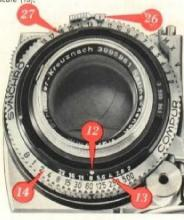
Even when you have set the exposure in this way, you can use the operture-speed coupling to adjust either the operture or the speed at will by turning the ring.
