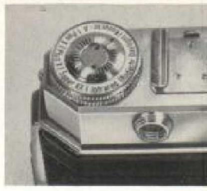
note: When the figure 1 in the film counter reaches the index, the film lever will lock; no more pictures can be made until the film is rewound into the magazine (see page 17) and the camera is reloaded. If the film lever locks at any time, do not force it but check the counter to see if it is set at 1. Move the counter off 1 to release the film winding mechanism.
