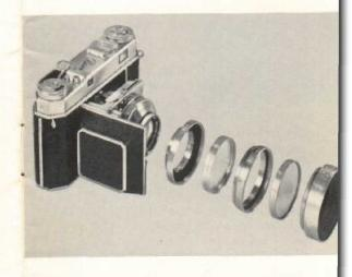
To assemble a filter, Portra Lens, or Kodak Close-Up Diffusion Disk in the ring, unscrew and remove the insert; then place the item in the ring; replace the insert. The Kodak Lens Hood can be used in place of the insert. If a Portra Lens and a filter or a Pola-Screen are to be used together, a Kodak Retaining Ring is also necessary.
