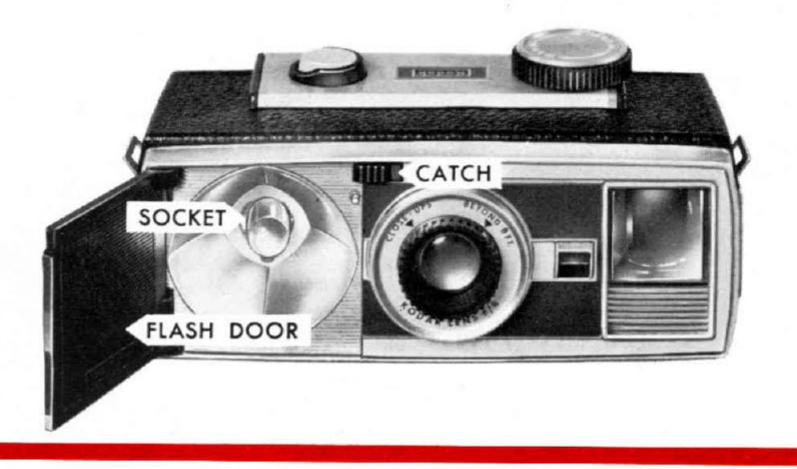
3 The distance from the camera to the subject is important for proper exposure. Keep within the distances in the table on page 10 and adjust the focusing mount for CLOSE-UPS or BEYOND 8 feet, depending on the camera-to-subject distance. Adjusting the focusing mount automatically selects the correct lens opening for flash.
