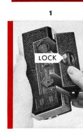
cover lock clockwise, as far as it will go (1/4-turn) to secure it in place. Check to make certain that the cover is fastened.
