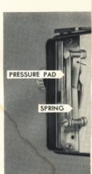
pad with a slightly moist cloth; do not scrape the track with any metallic object. Then polish the parts with a clean, soft, lintless cloth. Make sure the parts are dry.
