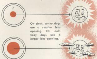
The lens opening marked 2.7 is the largest and admits the most light. Each succeeding marked opening from 2.7 to 16 lets through only one half as much light. Each marked lens opening is called a "stop"; the white dot between marked openings indicates a half stop.
