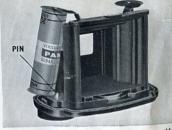
the paper, when unsealed, will unwind towards the picture aperture from the side of the spool away from the film holder. Engage the hole in the end of the spool with the pin on the spring. Push the spool up against the spring, and swing the spool into the recess until the hole at the other end engages the fixed lower pin.
