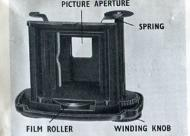
the spring. Now swing in the lower end of the spool, while turning the winding knob, and thus engage the winding key with the slotted hole in the spool.
