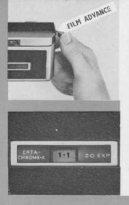
Push the FILM ADVANCE lever toward the front of the camera and allow it to return. Repeat until the lever locks—about a dozen full strokes (as the film advances, a series of arrows appears in the window). You are now ready for the first picture. After each picture, operate the film advance until it locks  $(1\frac{1}{2}$  to 2 strokes).
