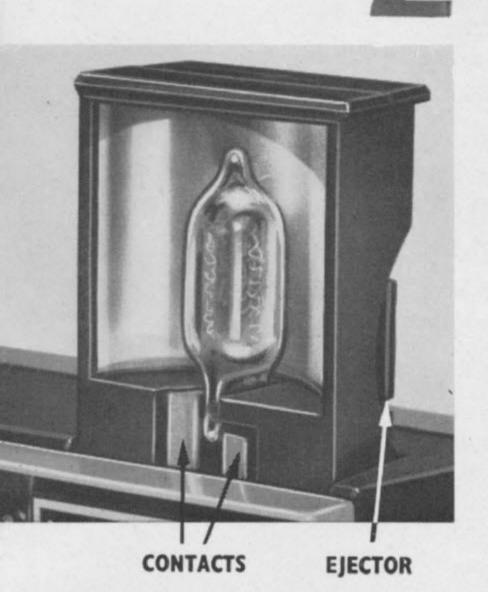
Insert an AG-type flashbulb by sliding the narrow edge of the glass base in between the Flasholder CONTACTS and pressing it back against the ejector finger until it is locked in place. To release a bulb, press the bulb EJECTOR as far as it will go toward the centre of the camera. Do not touch bulbs during or after firing – they will be extremely hot.
