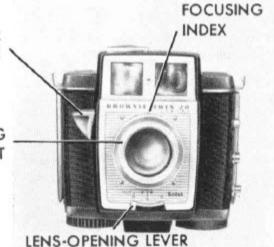
1 Set the LENS OPENING LEVER by moving it to the proper exposure value number. Make sure that the lever "click-stops" at one of the three numbers, not between them.
