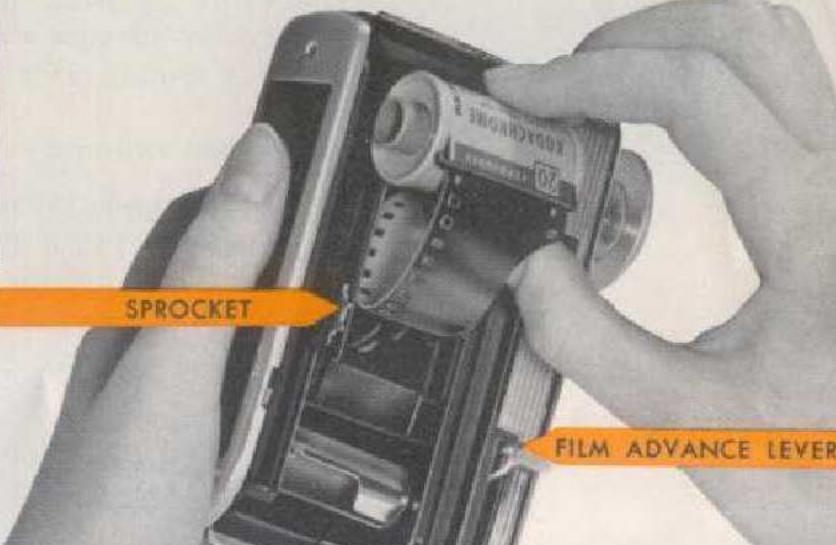
Drop the end of the film into the slot in the take-up drum. Hold down the edge of the magazine and move the film advance lever until the film is once around the drum. Close the back. Make sure it snaps in place. Move the film advance lever until the mechanism locks—this may require several full strokes of the lever.
